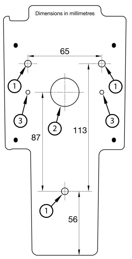
NOTE: Fix bracket to wedge before fitting to wall
